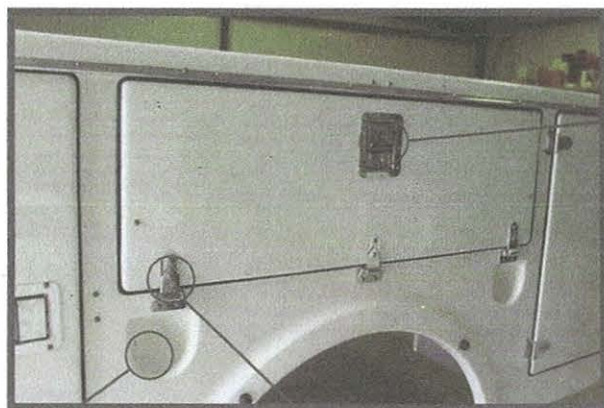
Stainless steel latches with optional remote key-less entry.
